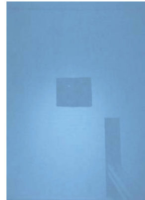
Figure 1. Ghost image (reflection) of the camera and camera support in the transparent cover plate. The target behind the cover plate is matt white paper.
