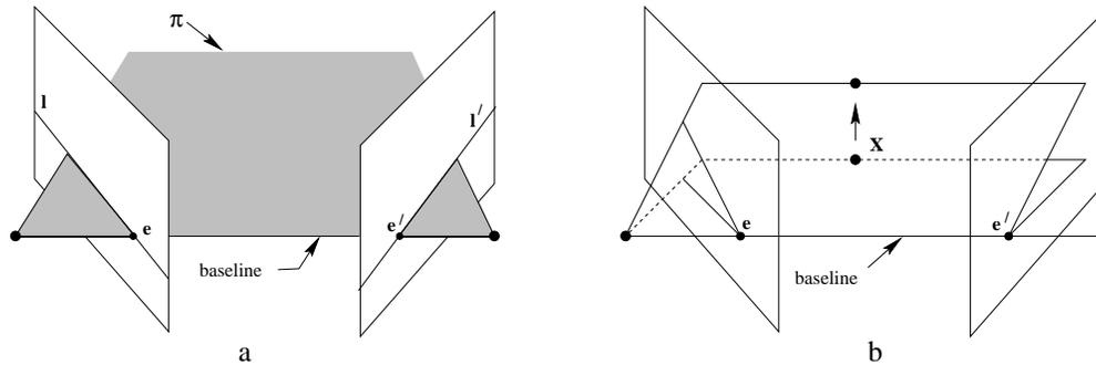
Fig. 9.2. **Epipolar geometry.** (a) The camera baseline intersects each image plane at the epipoles  $e$  and  $e'$ . Any plane  $\pi$  containing the baseline is an epipolar plane, and intersects the image planes in corresponding epipolar lines  $l$  and  $l'$ . (b) As the position of the 3D point  $X$  varies, the epipolar planes "rotate" about the baseline. This family of planes is known as an epipolar pencil. All epipolar lines intersect at the epipole.
