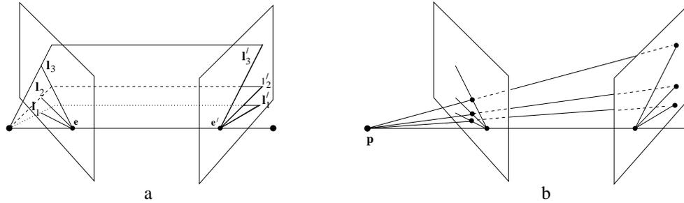
Fig. 9.6. **Epipolar line homography.** (a) There is a pencil of epipolar lines in each image centred on the epipole. The correspondence between epipolar lines,  $l_i \leftrightarrow l'_i$ , is defined by the pencil of planes with axis the baseline. (b) The corresponding lines are related by a perspectivity with centre any point  $p$  on the baseline. It follows that the correspondence between epipolar lines in the pencils is a 1D homography.
