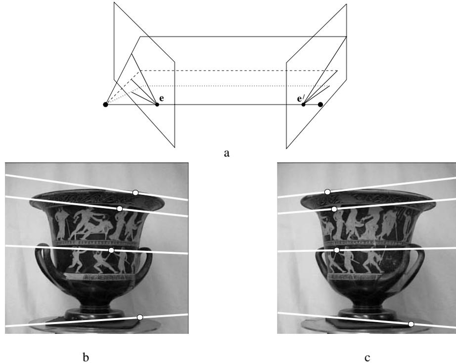
Fig. 9.3. **Converging cameras.** (a) Epipolar geometry for converging cameras. (b) and (c) A pair of images with superimposed corresponding points and their epipolar lines (in white). The motion between the views is a translation and rotation. In each image, the direction of the other camera may be inferred from the intersection of the pencil of epipolar lines. In this case, both epipoles lie outside of the visible image.
