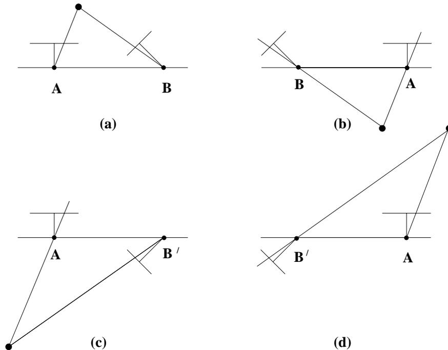
Fig. 9.12. **The four possible solutions for calibrated reconstruction from E.** Between the left and right sides there is a baseline reversal. Between the top and bottom rows camera B rotates  $180^\circ$  about the baseline. Note, only in (a) is the reconstructed point in front of both cameras.
