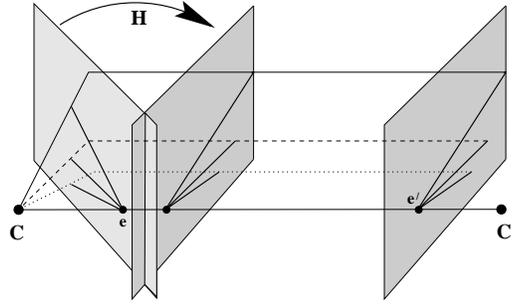
Fig. 9.9. **General camera motion.** The first camera (on the left) may be rotated and corrected to simulate a pure translational motion. The fundamental matrix for the original pair is the product  $F = [e']_{\times} H$ , where  $[e']_{\times}$  is the fundamental matrix of the translation, and  $H$  is the projective transformation corresponding to the correction of the first camera.
