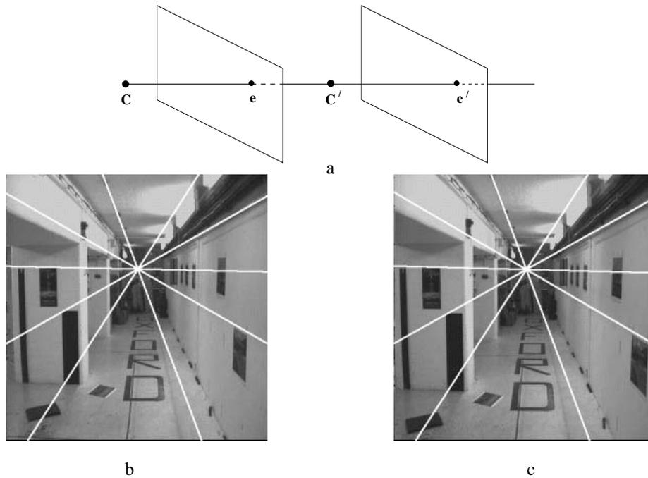
Fig. 9.8. **Pure translational motion.** (a) under the motion the epipole is a fixed point, i.e. has the same coordinates in both images, and points appear to move along lines radiating from the epipole. The epipole in this case is termed the Focus of Expansion (FOE). (b) and (c) the same epipolar lines are overlaid in both cases. Note the motion of the posters on the wall which slide along the epipolar line.
