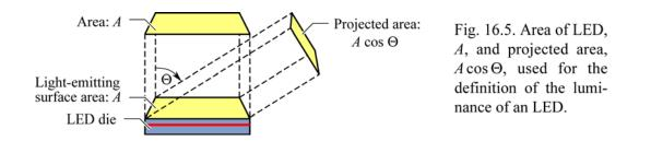
For LEDs, it is desirable to maximize luminous intensity and luminous flux while keeping the LED chip area minimal. Thus the luminance is a measure of how efficiently the valuable semiconductor wafer area is used to attain, at a given injection current, a certain luminous intensity.
