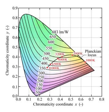
Fig. 16.8. Relation of maximum possible luminous efficacy (lumens per optical watt) and chromaticity in the CIE 1931 x, y chromaticity diagram (adapted from MacAdam, 1950).
