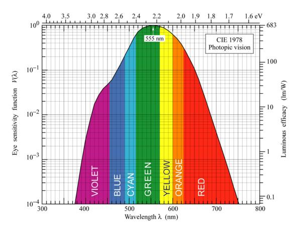
Fig. 16.7. Eye sensitivity function,  $V(\lambda)$ , (left-hand ordinate) and luminous efficacy, measured in lumens per watt of optical power (right-hand ordinate).  $V(\lambda)$  is maximum at 555 nm (after 1978 CIE data).
